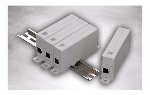
Used for IEEE 802.3af compliant networks which apply 48V power on pins 1, 2, 3, 6. Shielded RJ45 connectors are used and are bonded to protector ground. The unit has been designed to withstand 230Vac, common mode.
